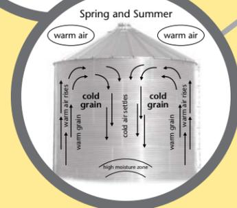
The aeration system and fan horsepower have to be adequate for the volume and configuration of canola storage. Also remember that the small size and round shape of canola seed leaves fewer air pockets relative to wheat and other larger grains, which adds to the aeration capacity requirement. For example, a 2,000-bushel hopper bottom bin may require only a 3 hp fan for wheat but will need a 5 hp fan to effectively condition canola.
