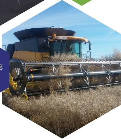
Figure 20. Crop bunching between reel and auger
