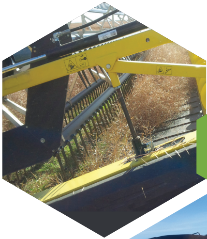
Figure 19. Draper header showing cross auger
