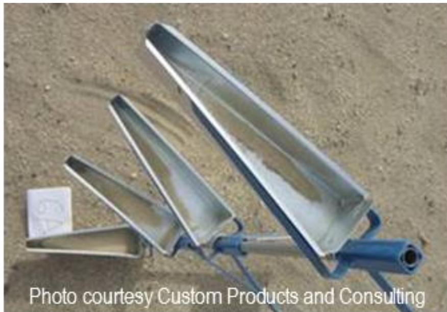
**Fig. 2.** BSNE soil samplers used to collect soil particles of varying sizes to determine potential dispersal of *Plasmodiophora brassicae* resting spores with wind erosion.
