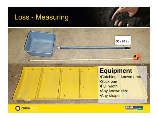
The you need to be able to catch material discharged from you combine. We refer to this as the catch pan. The only real requirement is that you know the area of the pan. Smaller pans of about 1ft square are easier to handle while large pans provide a more representative sample.
