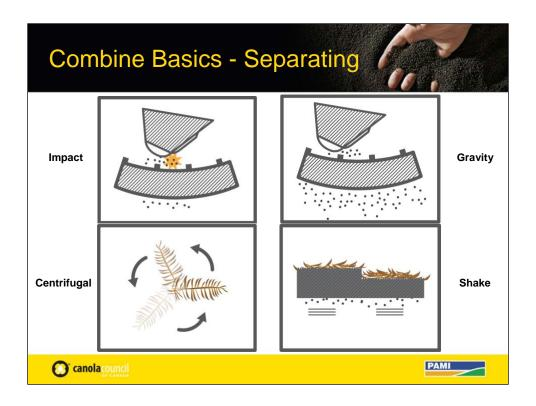
Separating has several factors that can assist grain on its way. The include impact, gravity, centrifugal and shaking
