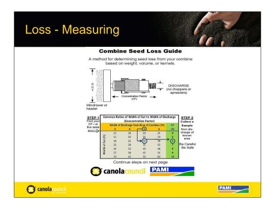
The loss guide provides simple steps to help you find a loss value. The first step is to recognize how much material has been concentrated into the width of the combine's discharge. The example shows that for a discharge width of 5 ft in the column below at 31 ft of cut the ratio is closest to 6 times. This can also be calculated by dividing the cut width of 30 ft by the discharge width of 5 ft which equals a ratio of 6.
