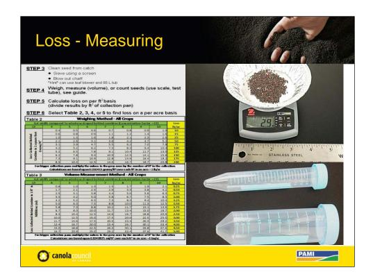
The measured loss now has to be converted to a loss per square foot. If your pan was 1 sq ft then simply look for that number under the column with the closes concentration number, in this case 6. If the pan was 4 square feet, then the weight or volume needs to be divided by 4.
