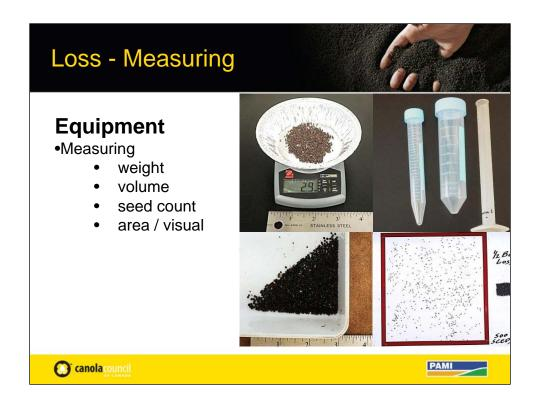
Measuring loss means establishing a quantitative amount. There are various means including weighing, volume in a marked container, and area (visual) and seed count which is not practical for canola when loss is not close to negligable.
