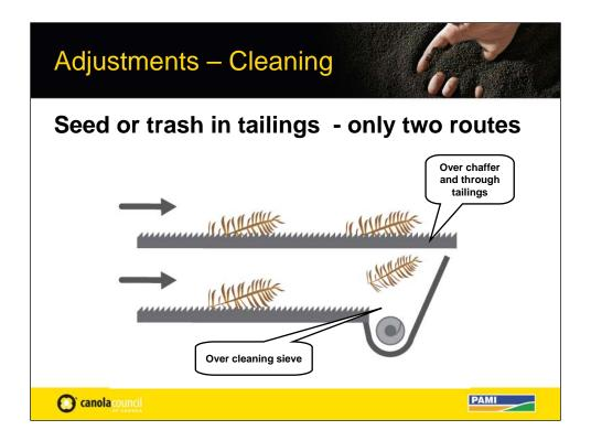
An overloaded tailings whether it is trash (chaff) or grain you need to identify how it got there so that you can address it with the proper adjustment. There are only two ways, it travels over the chaffer sieve and falls through the tailings sieve or it falls through the chafer sieve and travels over the cleaning sieve and dumps into the tailings. Close the tailings sieve off to determine which route it is following.
