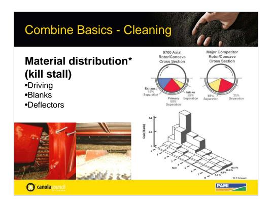
All cleaning systems are sensitive to crop distribution that includes the grain and the chaff, especially as how the distribution aligns with air distribution. This might be a result of driving, feeding or machine design. The kill stall works well for most rotary combines. This means stopping the combine as quickly as possible under load.
