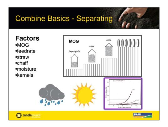
Some of the most influential factors that effect separation include MOG/G ratio, MOG feedrate, straw condition , chaff, moisture and kernel characteristics
