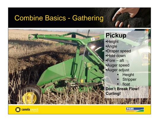
Even a uniform windrow is no guarantee of uniform feeding. Pickup adjustment can significantly effect crop feeding. Adjustments such as pick-up Angle, picking and transfer belt speed, auger speed, auger finger timing, auger height and fore-aft adjustment, auger stripper position and adjustment, auger float and auger flighting all can cause breaks in other wise uniform crop flow.
