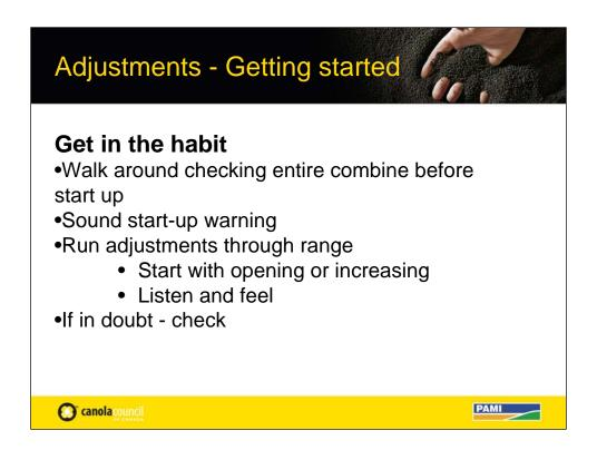
Before adjusting it is wise to develop a routine that eliminates issues before they become problems. Check your combine before start up to ensure all doors are shut and access panels are in place. Make sure there are no mechanical issues such as loose hangers, damages belts or chains, missing parts etc. look for plugged components and anything that appears out of the ordinary.
