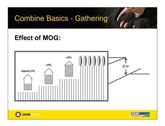
Combine capacity is generally a factor of the MOG that is taken in with the grain. As such reducing the straw means you get to go faster to reach the critical MOG throughput. This means a higher grain capacity.
