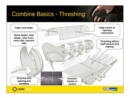
There are many mechanical factors that effect threshing. Everything from the rotor impellers to the concaves. Rotor cage vanes and cage covers or interrupters can effect threshing just as the concave design and concave blanks can. Threshing ultimately effects the amount of chaff and the makeup of the chaff. threshing
