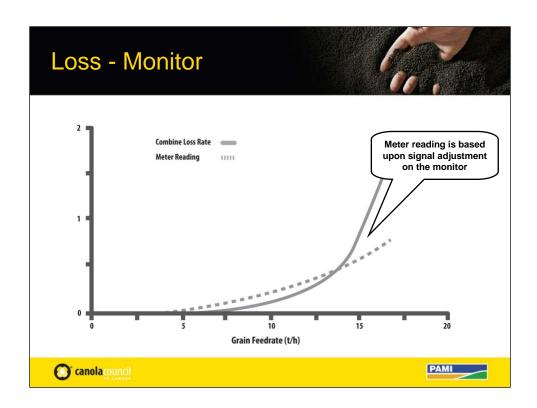
Loss and loss monitors have been inextricably ties together. Loss monitors must be calibrated to be at all useful. Still they can fool you!
