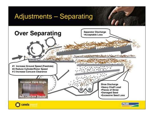
Is there such a thing as over separating? You can't save too much grain but you can separate too much chaff, to the point where it effects cleaning. Normal adjustment might include increasing feedrate, slowing the cylinder/rotor speed and opening the concave. I may also include changing to narrow wire spaced concaves, blanking portions of the concaves or separating grates or advancing the cage vanes.
