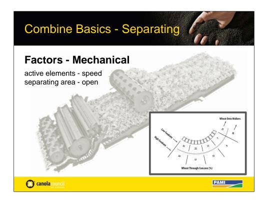
Separation is most efficient when under active elements such as cylinder and concave. It is important to recognize that separation is highest when the grain to MOG ratio is highest and the crop is moving slowly.
