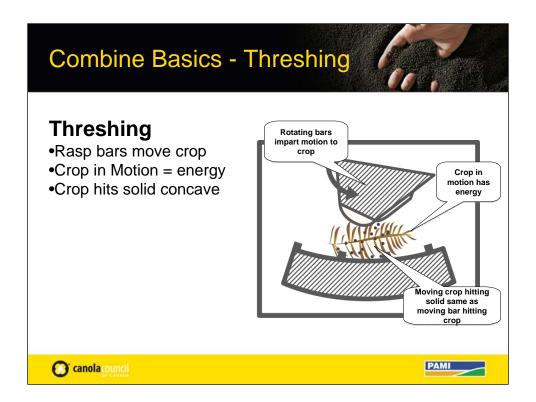
We know there is energy transfer when the fast moving bars contact the slow moving crop. We also know that when the crop flows and crashes into a stationary bar again energy is transferred to threshing the seed from the head or pods.
