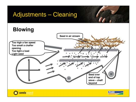
The cleaning shoe can loose grain in several different manners. One way is referred to as "blowing" seed over. It is characterized by the seed dropping off the end of the top sieve but the chaff is blown above and beyond. This basically happens when there is too high an air velocity. This causes grain to travel over the top sieve without falling through.
