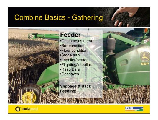
If crop flows smoothly to the feeder there is still a chance that it will slip or bunch due to improper chain adjustment, poor feeder bar condition, rust or dirt on the feeder floor, obstructions in the stone trap, worn beater or impeller wings, or the wrong ones for the crop, worn rotor impeller fins or infeed flighting, worn rasp bars or concave inlet obstruction can cause uneven material flow.
