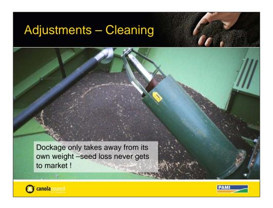
Cleaning the sample to the desired level tends to be individual preference but running too much clean grain through the tailings usually results in extra seed damage, and you might only ever see half of the damage if at all. So far dockage is just subtracting junk from its own weight so you are not out anything.
