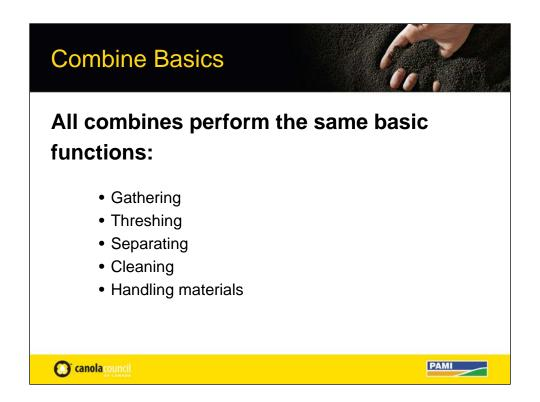
All combines perform the same basic functions of Gathering which is getting the crop into the combine, Threshing to dislodge the seed from the plant, separating to get the seed removed from the main stems, cleaning which captures the seed separate from the chaff and material handling that moves the seed to the holding tank and from the combine to an exit point and includes moving tailings and conveying straw and chaff which often is chopped and spread.
