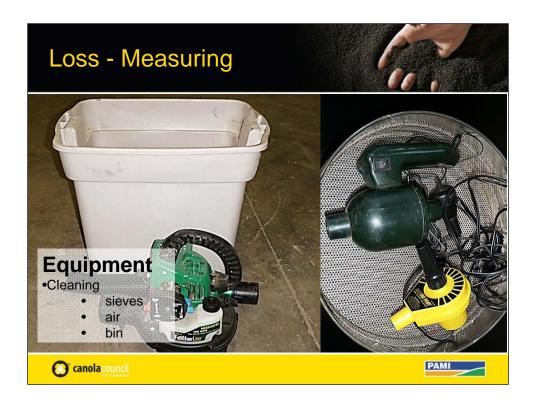
Once you catch a sample you have to get to the clean seed. Cleaning is made easier if you have (dockage) screens and some portable fan to blow out chaff and dirt. For large samples you can go to a tub and leaf blower or even a portable cleaner (Clipper fanning mill)
