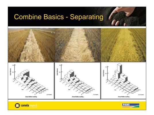
Uniform head distribution provides optimum separation at the concave and walkers. Concentrating the heads either in the middle or at the side and separation limits are reached sooner than at the rest of the available area. The result is much higher loss at the same overall feedrate.
