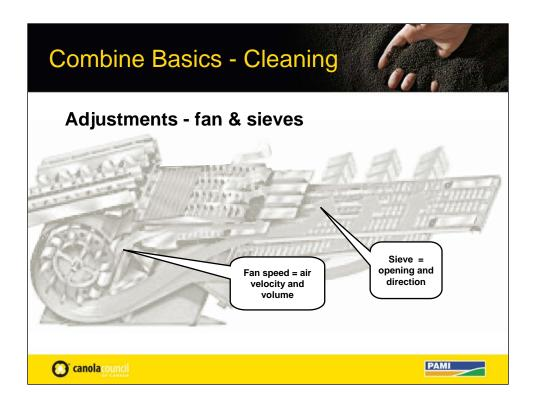
The fan provides the air velocity and volume (higher velocity = higher volume). The sieves provide and perforated medium that has mechanical conveyance and tossing and the opening also provides air direction control.
