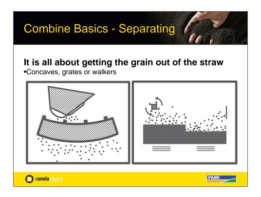
Once threshing starts to take place, separation also starts. Threshing keeps the MOG on one side of a medium and grain passes through.
