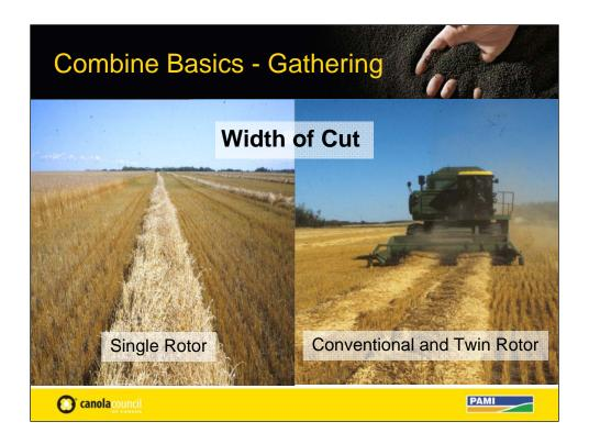
Single axial rotor combines prefer narrower windrows due to limited feeder width and in-feed challenges at the rotor. Conventional (wide cylinders) and twin rotors like wider windrows to spread out crop across cylinder width and to provide separate streams to each of the twin rotors especially like the loose center.
