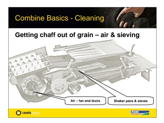
There are two main mechanical features that effect cleaning they are the air and the sieves.
