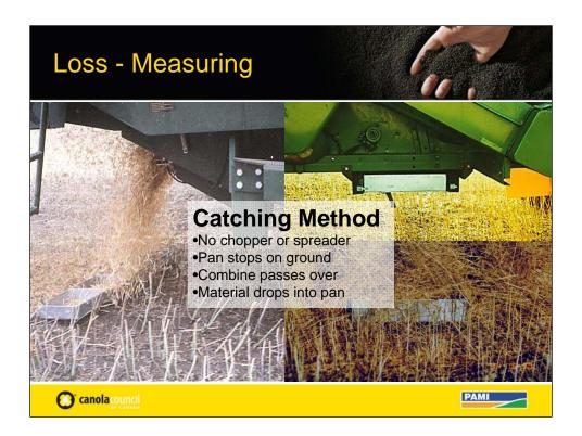
For loss collections to provide reasonable representation the combine's straw and chaff choppers/spreaders must be out of the way so that the combine discharges directly onto the ground. The pan must be placed ahead of where the discharge will land so that as the combine moves forward the discharge lands in the pan.
