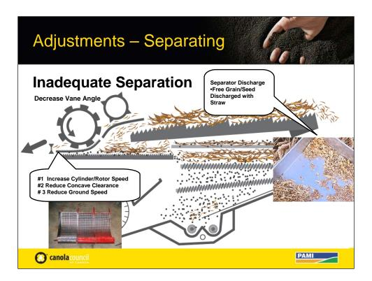
Inadequate separation simply means too much separator loss! You can choose to increase threshing settings based upon threshing results. This means increasing cylinder/rotor speed, decreasing concave clearance or decreasing feedrate. If these aren't desirable options increase concave separating open area by changing to wide spaced wire concaves or pulling wires. Another option is decrease the concave age vane angle .
