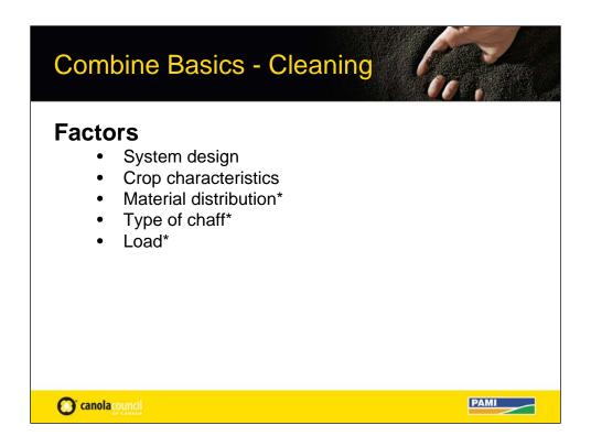
Every cleaning system is subject to the integrity and efficiency of its design —some good — some not. Each system may respond differently to changing crop characteristics and conditions. All systems are effected by uneven material distribution. Cleaning systems are chaff dependent not only as a function of load but also by the chaff composition and characteristics.
