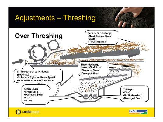
When over threshing is the problem and losses are not a problem then drive a faster. Typically however, the worst problem will be either grain damage or unthreshed. In his case increase cylinder/rotor speed, followed by tighter concave clearance.
