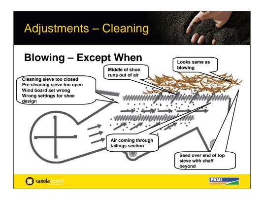
When is blowing not blowing? It may look like blowing but the reason the grain is getting to the back is because it has settled onto the top sieve and rode back. This may be from a loss of air in the mid section of the top chaffer sieve due to the precleaner being too far open, the bottome cleaning sieve closed too much a windboard set incorrectly or poor design.
