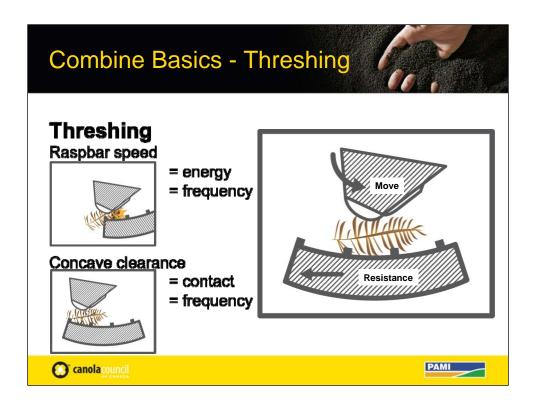
We know that threshing bar speed inputs the energy and also determines the frequency the bars pass a given point that affects the odds of crop being impacted. The concave provides restriction to crop flow as well as the anvil to hammer the crop against. Increased resistance also will increase the frequency of contact.
