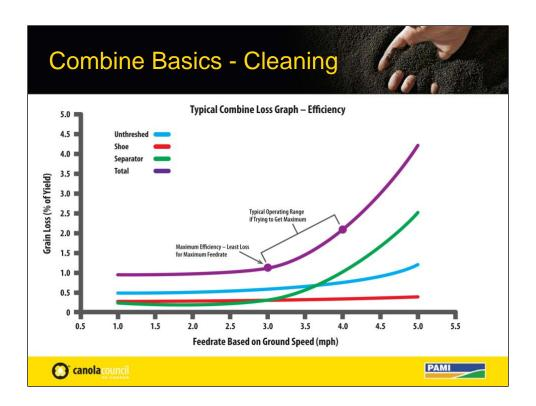
Cleaning systems tend to be chaff feedrate dependent. Eventually as feedrate increases it becomes less efficient and begins loosing seed. In the worst case, an overloaded system will fail to function and seed pours over.
