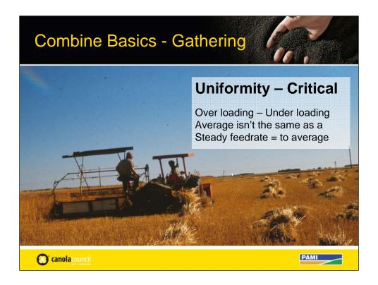
The more uniform the crop flow the better the combine will perform. A wide variation in feedrate will not produce a same average feedrate as when feeding is very uniform. Once a combine's system is overloaded, it takes time to recover and under loading can not be adjusted for quickly enough for variations occurring over a short distance.
